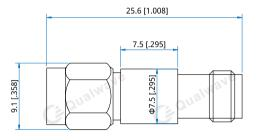
Unit: mm [in] Tolerance: ±3%
